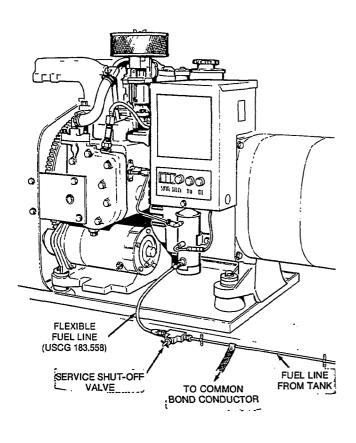
FIGURE 7. FUEL SHUT-OFF VALVE
