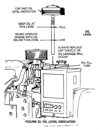
The engine oil capacity is 3.5 quarts (3.3 litre). Do not overfill crankcase. Engine oil should be drained when warm at recommended interval shown in Table 1. Remove the oil base drain plug, or if preferred, pump the oil out through the oil fill tube.
