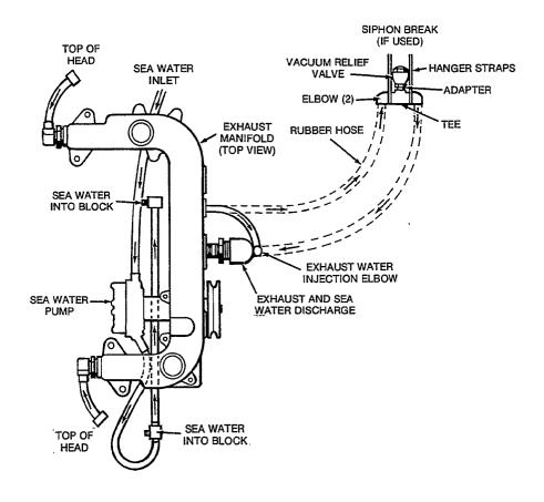
FIGURE 10. HOSE SCHEMATIC, SEA WATER COOLING
