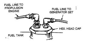
FIGURE 5. TWO FUEL LINES IN ONE TANK OUTLET
