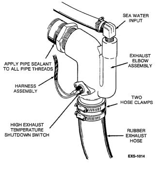
FIGURE 8. SEA WATER CONNECTIONS
