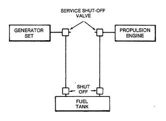
FIGURE 4. ABOVE TANK LEVEL INSTALLATION
